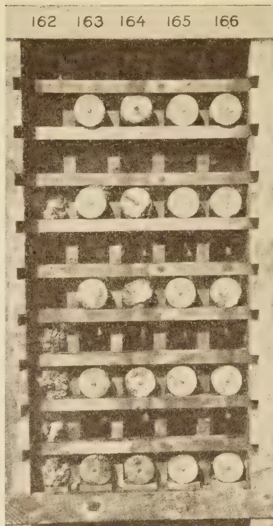
Cylinders with calcium chloride admixed in following proportions, after six years in lake: Series 162.—4 per cent Series 163.—8 per cent Series 164.—4 per cent Series 165.—8 per cent (cured in water vapor at 155° F., 48 hrs.) Series 166.—4 per cent (cured in water vapor at 155° F., 48 hrs.)
